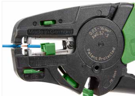
Partially stripping a conductor.
