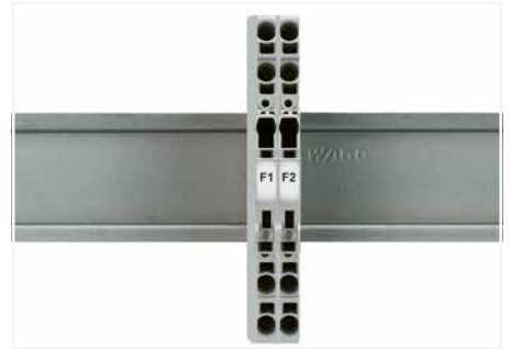
Fuse terminal blocks with a width of 6.2 mm can be assembled adjacently. If there is no adjacent fuse terminal block at the end of the assembly, an end plate must be used.
