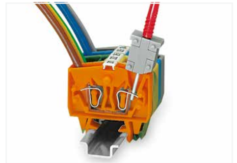
Testing via CAGE CLAMP® on the current bar (max. nominal current: 6 A) – CAGE CLAMP® clamps individual test contacts. The maximum test voltage is 400 V.
