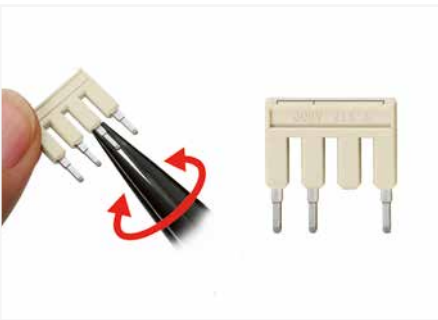
Custom jumpers are created by breaking and removing jumper contacts (2000, 2001, 2002, 2004 Series).
