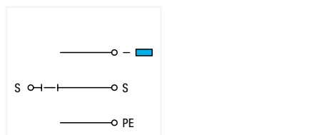
Actuator disconnect terminal block; with ground connection; for phase interruption
