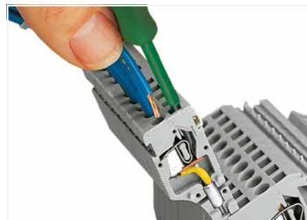
CAGE CLAMP® connection 0.08 ... 1.5 mm 2 ; 5 mm wide module 0.08 ... 2.5 mm 2 ; 6 mm wide module
