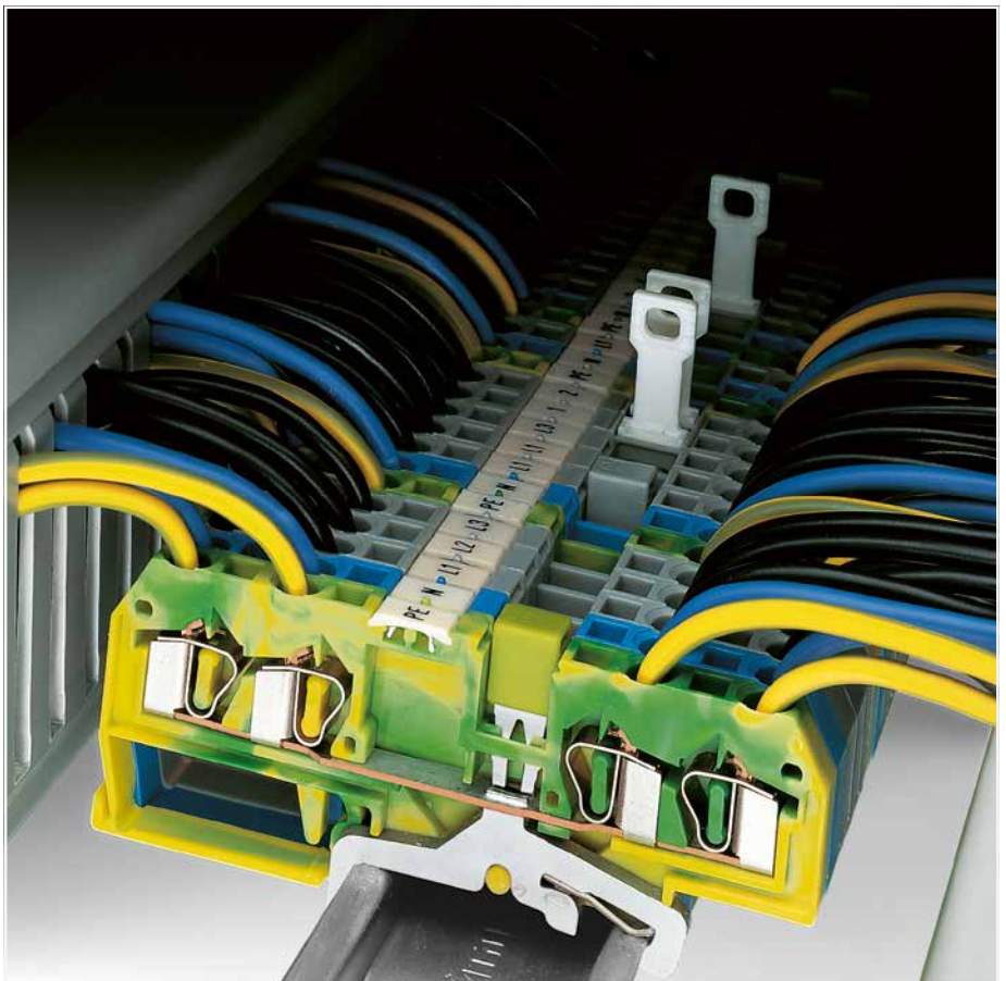
Steel DIN-rails are not suited for PEN (ground and N-conductor) applications per EN 60947-7-2 (VDE 0611, Part 3).
