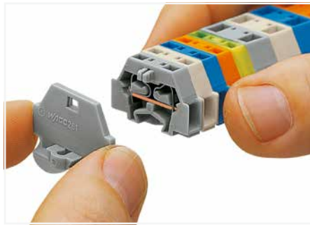
Mounting an end plate.
