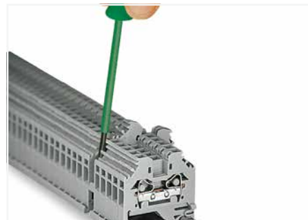
Removing a terminal block from the assembly.
