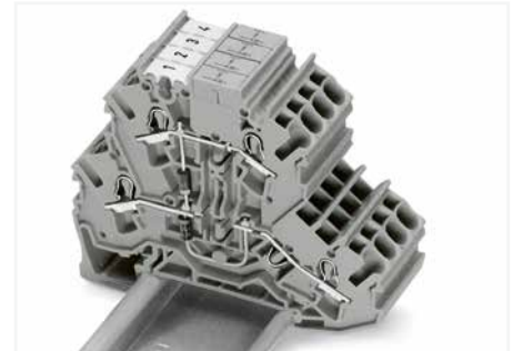
Double-deck diode terminal blocks were specifically developed for custom diode circuits, such as lamp test and collective fault signal circuits. These terminal blocks provide high-density wiring in a width of just 5.2 mm. Push-in type jumper bars provide additional options for custom circuit design.
