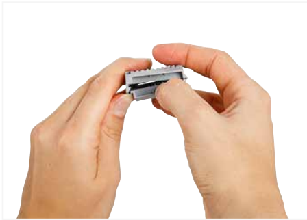
Open the Gelbox at the side latches.
