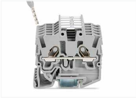
Insert ferruled conductors via push-in termination.
