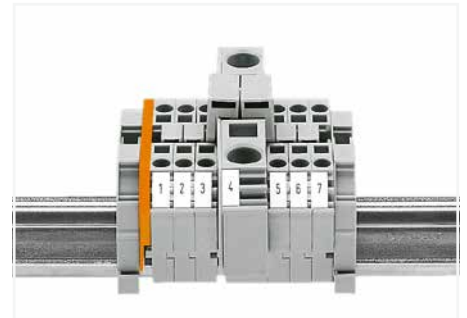
Commoning from 16 mm 2 /6 AWG (283 Series) to 4 mm 2 /12 AWG (281 Series) rail-mount terminal blocks via step-down jumpers.
