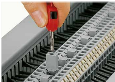
Testing with a test plug – Picture shows a test plug adapter (209-170).
