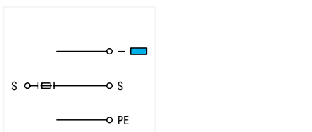
Actuator terminal block; with ground connection; for fuse plugs; for phase protection; without end plate
