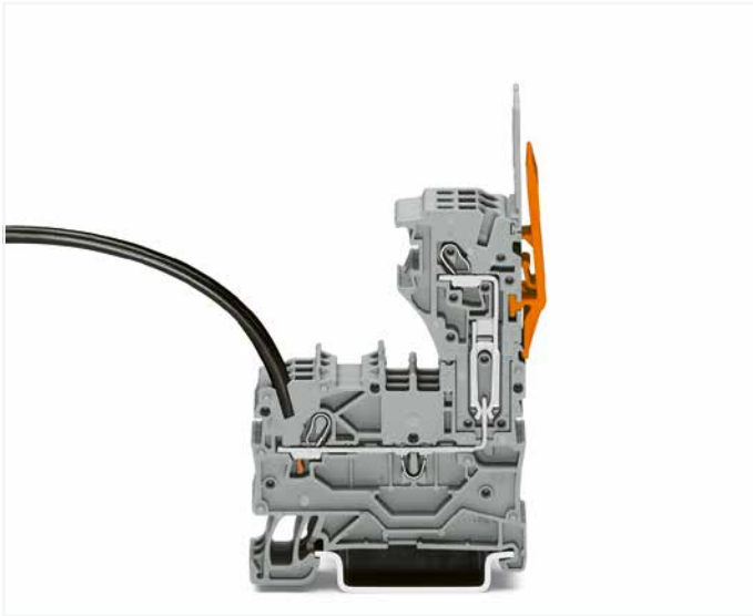
1-conductor female plug Carrier terminal blocks can be commoned via 2000 Series Push-In Type Jumper Bars and tested via 859-500 Test Pin.
