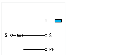
Actuator terminal block; with ground connection; for fuse plugs; for phase protection; with end plate Terminal block width: 6 mm / 0.236 inch
