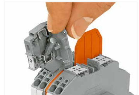
An end plate for fuse disconnect terminal blocks (shown in orange, 2002-1092) is used for additional protection, preventing the fuse holder from being opened. The fuse cannot be replaced until disconnecting the fuse holder from the power supply.
