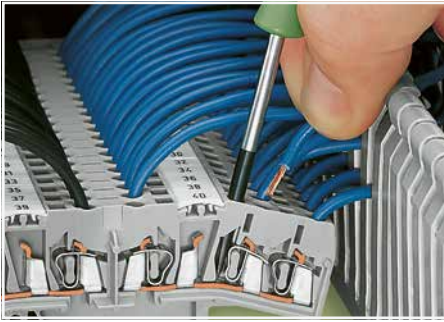
Terminal blocks for matrix patching: Inserting/removing a conductor on the terminal block's side-entry. With ferruled conductors, it is necessary to use a terminal block one size smaller than the conductor's nominal cross section.
