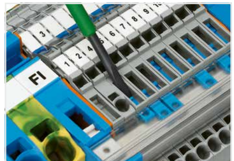
Operating a disconnect slide link with an operating tool (3.5 mm blade width) Item number (operating tool): 2009-309, 2009-310, 210-658 or 210-720
