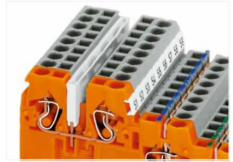
Commoning signal level voltage via insulated push-in type jumper bars (870 Series) – 2- to 9-way, depending on application. Sensor LED terminal blocks cannot be commoned!
