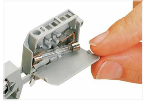
Fuse replacement: One end of the fuse is automatically ejected from the holder when opening the cover.
