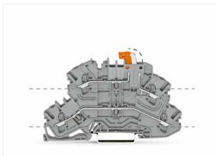
Double-deck disconnect terminal blocks with a pivoting knife disconnect (2002-2671) can be used as through terminal blocks on the lower deck and as disconnect terminal blocks on the upper deck. Besides disconnection and measurement, double-deck carrier terminal blocks (2002-2667) also provide ground conductor functionality.
