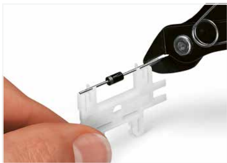
Cutting component to the proper length.
