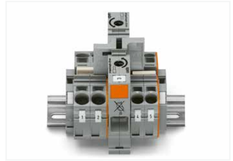
Commoning 35 mm² (2 AWG) POWER CAGE CLAMP Terminal Blocks with 10/16 mm² (8/6 AWG) 2010 and 2016 Series Terminal Blocks TOPJOB® S using step-down jumpers (not valid for 2016-76xx and 2016-77xx).
