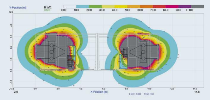
Magnetic field lines of an EMC calculation
