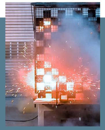
Internal arc fault test arrangement according to IAC-A 20 kA 1s for protection of operating staff
